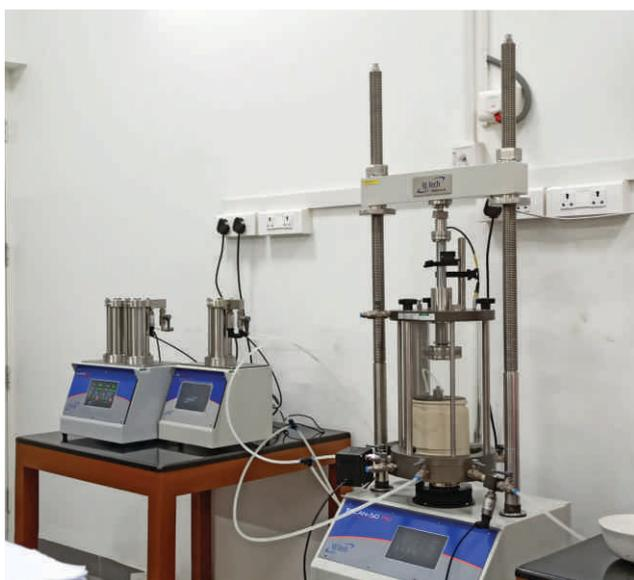
Automated stress-path static triaxial apparatus with permeability measurement
