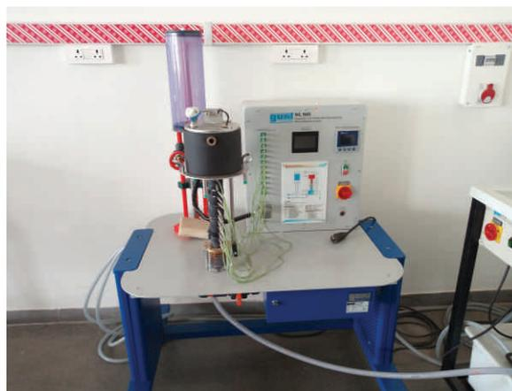
Thermal conductivity measurement setup
