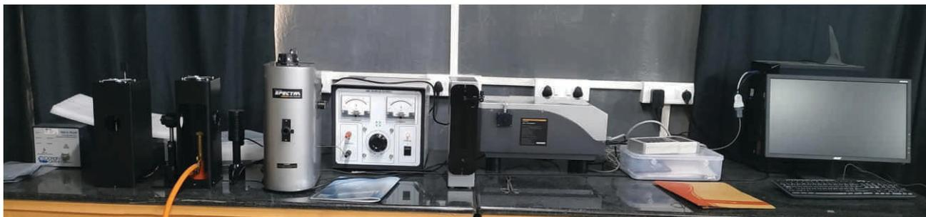
UV-VIS emission and absorption spectroscopy of gas and liquid phase systems
