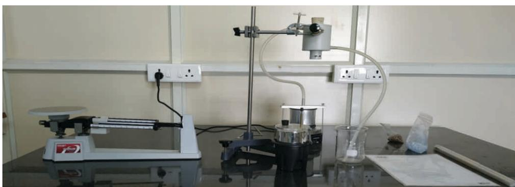
Apparatus to measure the heat capacity
