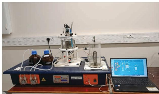
Continuous Stirred Tank Reactor
