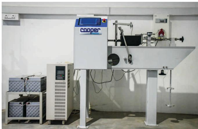
Automated direct shear apparatus
