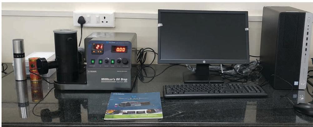
Millikan's Oil Drop apparatus to determine the charge of an electron
