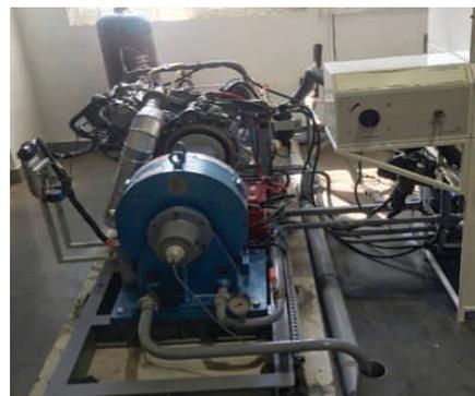
Two-cylinder CRDi Diesel engine setup
