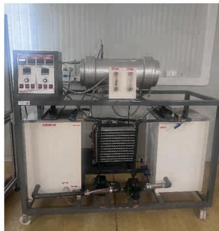
Shell and Tube Heat Exchange
