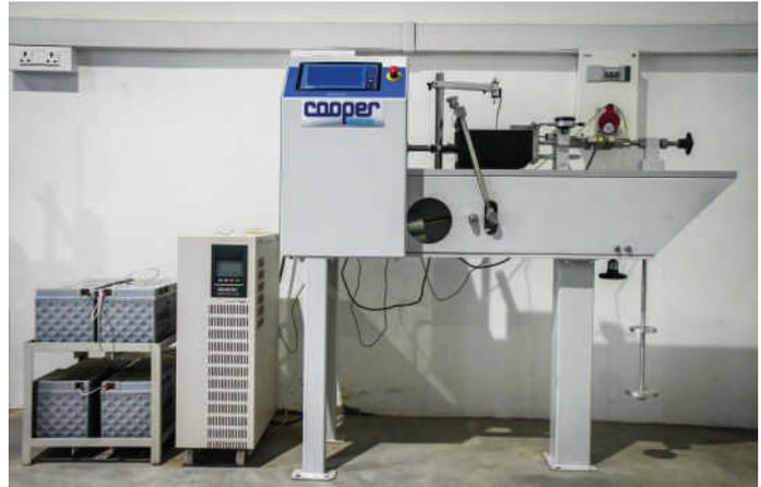
Automated direct shear apparatus
