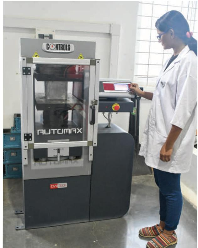
2000 kN Load controlled Compression Testing Machine
