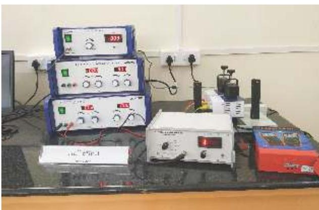
▲ Fig. 21 Hall effect apparatus for metals
