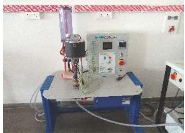
▲ Fig. 70 Thermal conductivity measurement setup
