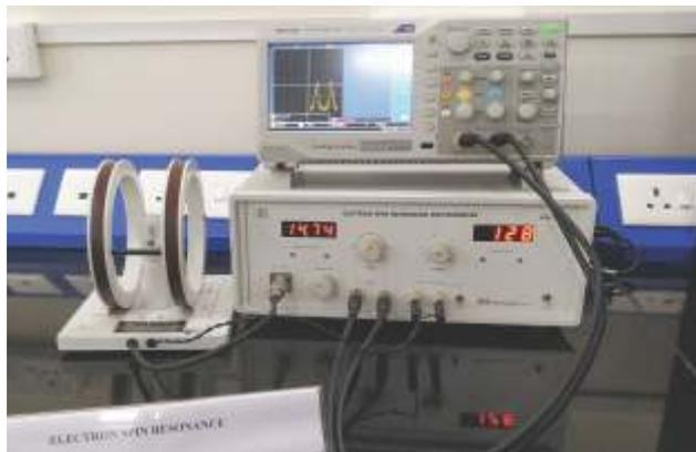
▲ Fig. 24 The Electron Spin Resonance (ESR) setup with Helmholtz coil and digital oscilloscope
