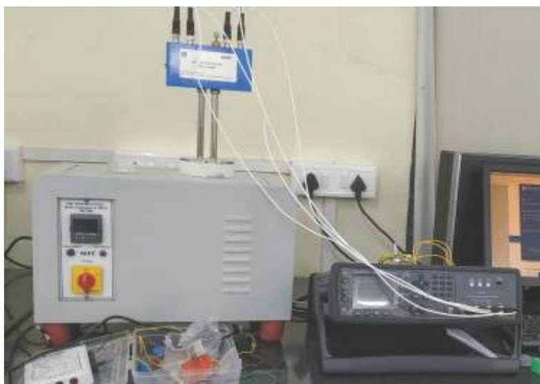
◀ Fig. 26 LCR meter for the dielectric constant measurement
