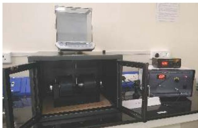
▲ Fig. 22 Gouy's balance for measurement of the magnetic susceptibility
