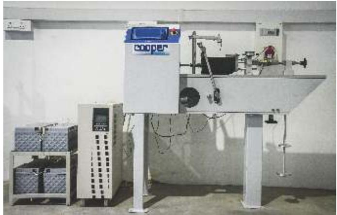
▲ Fig. 43. Automated direct shear apparatus
