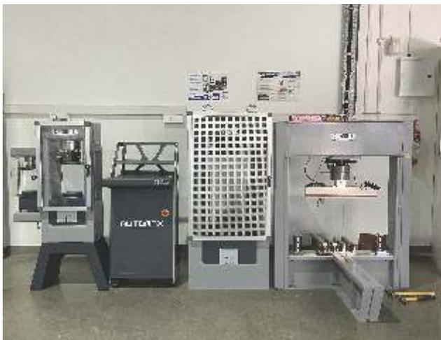
▲ Fig. 38 Family of Compressive Testing Machine
