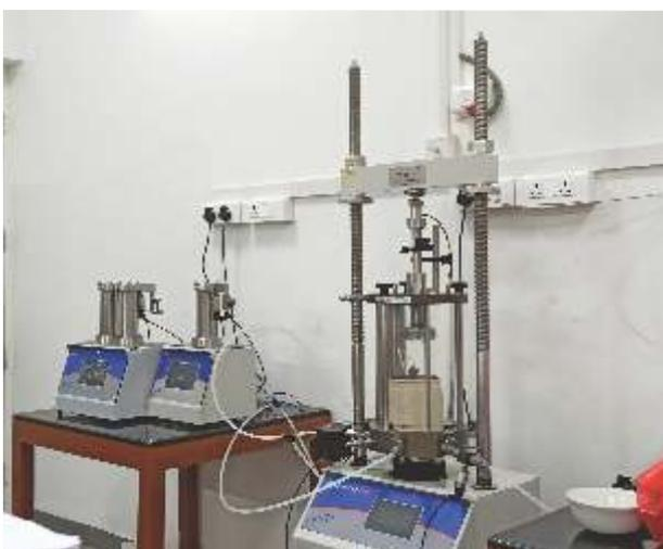
▲ Fig. 45. Automated stress-path static triaxial apparatus with permeability measurement
