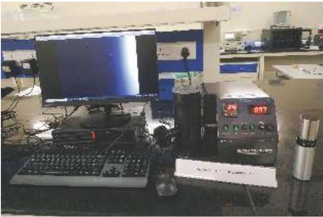
▲ Fig. 18 Millikan's Oil Drop apparatus to determine the charge of an electron
