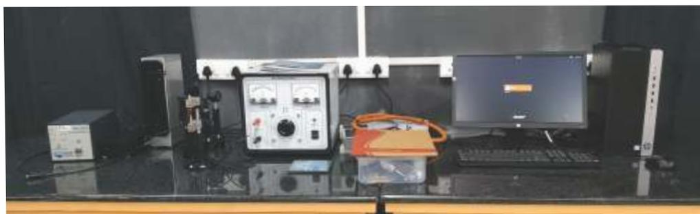
◀◀ Fig. 16 UV-VIS emission and absorption spectroscopy of gas and liquid phase systems
