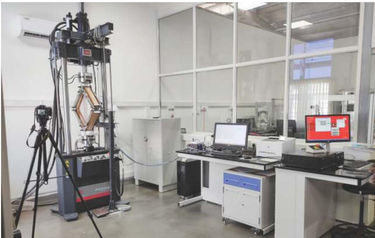
▲ Fig. 33 A view of lab with 100kN UTM and DAQ system
