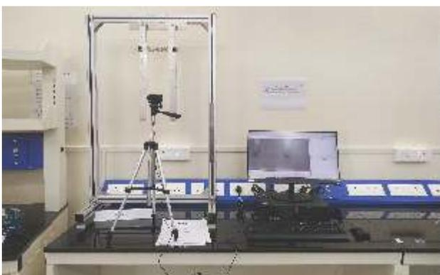
◀◀ Fig. 17 Coupled Pendulum setup along with a high-resolution camera
