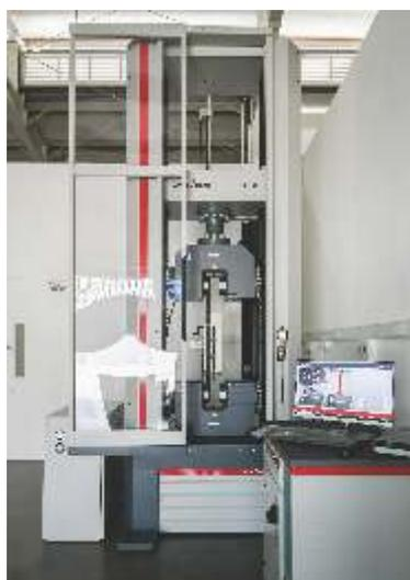
◀ Fig. 34 High capacity Electro-mechanical UTM in Structural Engg lab
