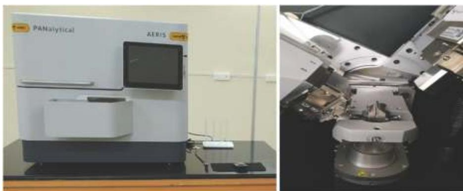
◀◀ Fig. 27 The Benchtop AERIS Panalytical X-ray diffractometer (Left), inner view of the diffractometer having the X-ray source, sample stage and detector (Right)
