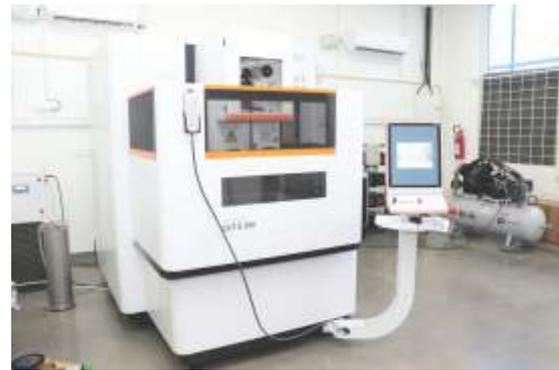
▲ Fig. 74 CNC WIRE CUT EDM
