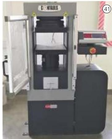
► Fig. 41. 2000 kN Load Controlled Compression Testing Machine
