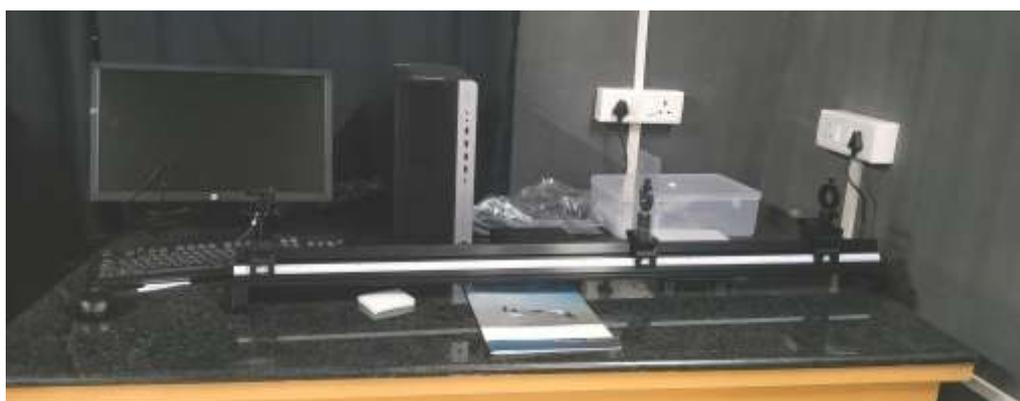
◀ Fig. 13 Single slit diffraction setup
