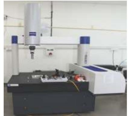
Fig. 71 Coordinate Measuring Machine
