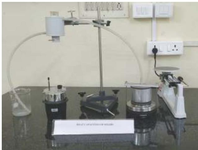
▲ Fig. 23 Apparatus to measure the heat capacity
